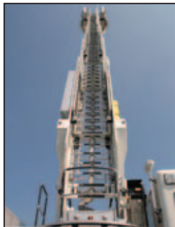
Clear ladder walkway for easier access
